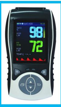
**Display screen** Type: 2.8 inch TFT coloo LCD Display area: 58mm×43 mm
