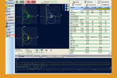
The PRO SPIRO N PC-Spirometer is dedicated for use on a PC or Notebook with USB connection. The operation and evaluation is performed by the computer. The use of bacterial / viral filters is recommended.
